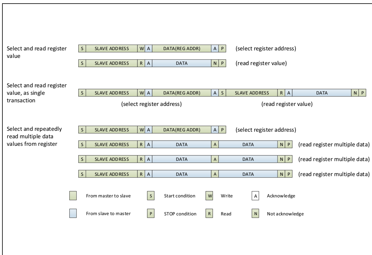
Figure 10: I 2 C Register Read
